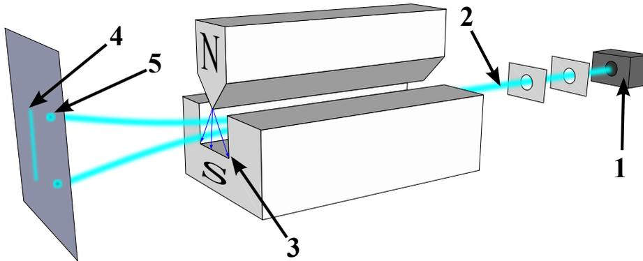
Figure 9.1: Setup of the Stern-Gerlach experiment. (1) furnace, (2) beam of silver atoms, (3) inhomogeneous magnetic field, (4) classically expected result, (5) observed result. Picture credit: [http://en.wikipedia.org/wiki/Stern-Gerlach\\_experiment](http://en.wikipedia.org/wiki/Stern-Gerlach_experiment)
