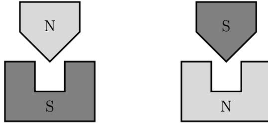
Figure 9.3: LEFT: Schematic picture of a Stern–Gerlach magnet. RIGHT: Modified Stern–Gerlach magnet with inverted polarity (north and south exchanged roles) while keeping the shape.
