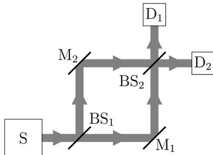
Figure 15.1: Design of a Mach–Zehnder experiment. Wave packets travel along grey paths in the direction indicated. S = source, BS = beam splitter, M = mirror, D = detector.
