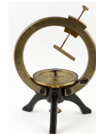
1986. Victor Goldschmidt two-circle contact goniometer
