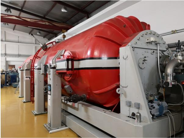
Figure 3: 6.0 MV EN Tandem Van de Graaf accelerator at RBI research facility.
