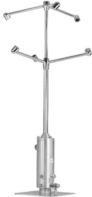
so as to get lower flow distortion. Also, sensors were developed, which can be used for all flow directions (omni-directional, Fig. 6.14). A problem yet to be investigated, is the significant self-correlation of the Cartesian wind components from the inclined wind components, which influences the statistical independence for the calculation of the covariances.
